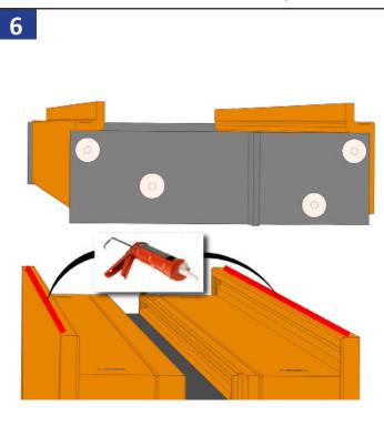
Apply two continuous beads of silicone on top of the first unit, the full length of the unit as shown. Set the stack mull on top of the first unit.
