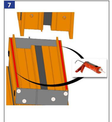
With the stack mull in place, apply two continuous beads of silicone on top of the mull along its full length as shown. Set the second unit on top of the stack mull.
