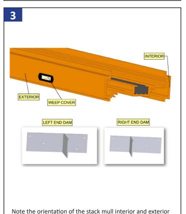
sides. Exterior side will have weep slots. Note orientation for
