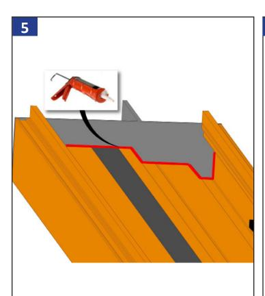
Apply a continuous bead of silicone along the entire inside of the edge of the end dam following the contour of the mull. Repeat for the other end.
