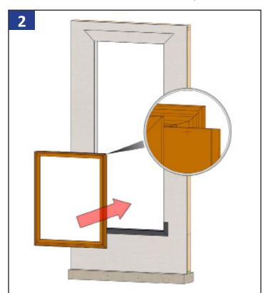
Install the bottom unit in place following the QWP standard nail fin installation guide. Check the unit has the nail fin removed on the top side where the stack mull will go.
